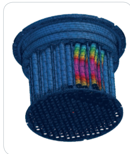
Large model of reactor vessel's upper internals from AREVA. (Simulation case using unrealistic loads) Courtesy: AREVA
