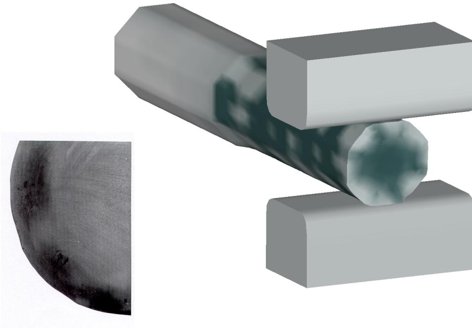
The final stage of cogging in a four-pass heat showing contours of grain size in billet (right). Darker shading represents finer grains. Note the eight pockets of coarse, un-recrystallized grains on the periphery.
