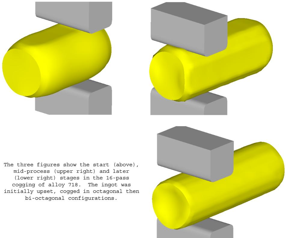
The three figures show the start (above), mid-process (upper right) and later (lower right) stages in the 16-pass cogging of alloy 718. The ingot was initially upset, cogged in octagonal then bi-octagonal configurations.
