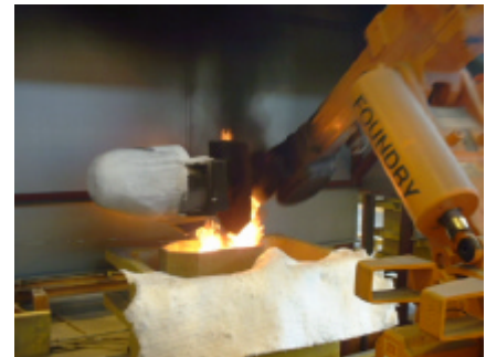
Figure 9: (left) The coated foam just before the vibration station. (Courtesy of Montupet)
