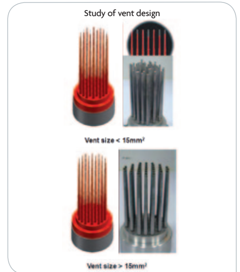
Smaller vent sizes reveal insufficient filling due to back pressure, while 100% filling is observed in dies with well designed vents.
