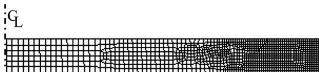
Fig. 6. Finite element mesh employed for the blank.
