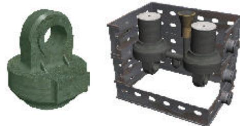
Figure 4: Steel casting part (68 Kg) and its position in the sand mold (Courtesy of DSB Blansko).
