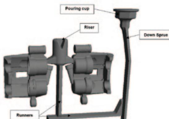
Filling System used to manufacture the part
