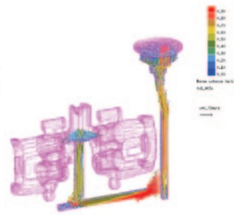
Mold cavity filling process with the different velocities reached by the liquid metal when entering the parts
