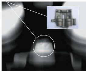
Areas with micro shrinkage defect
