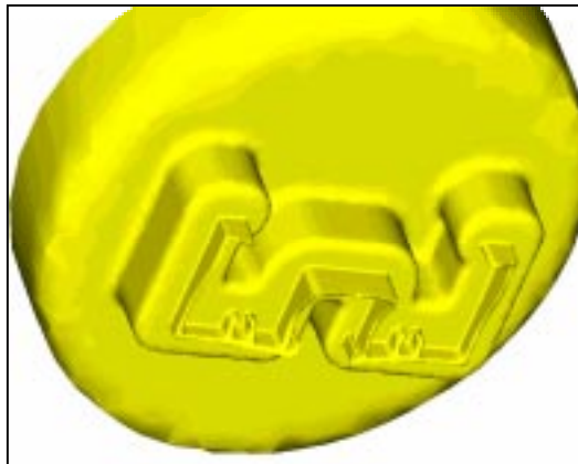
Figure 1 Above: The transient behaviour of the non-steady state condition is simulated showing the first metal to leave the die [1].
