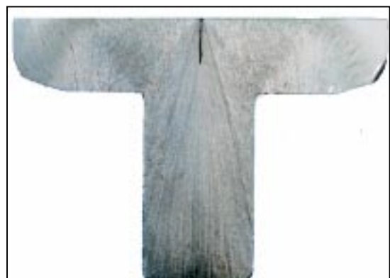
Figure 7 Right below: Piping defect encountered in the actual part [2].
