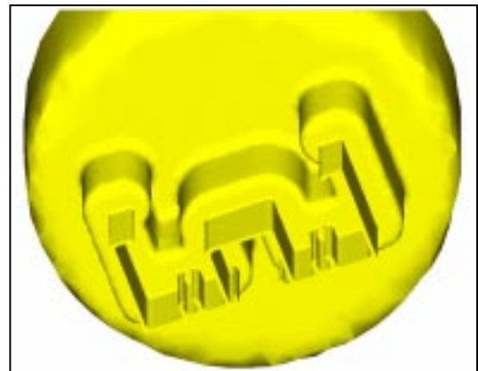
Figure 1 Above: The transient behaviour of the non-steady state condition is simulated showing the first metal to leave the die [1].
