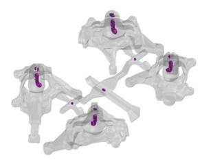
Shrinkage porosity map on four of the eight cavities of the new molding layout (symmetry considered during simulation with ESI QuikCAST)
