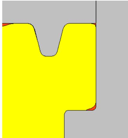
This image shows the last areas to fill in red. The underfilled regions (shown in red) fill the die cavity almost simultaneously.
