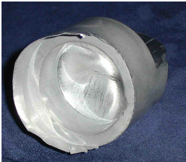
The piping area is shown as a dark horizontal mark directly under the punch face.
