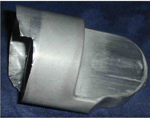
The part as extruded at JLO is shown. Note the flash on top (left) of the part.
