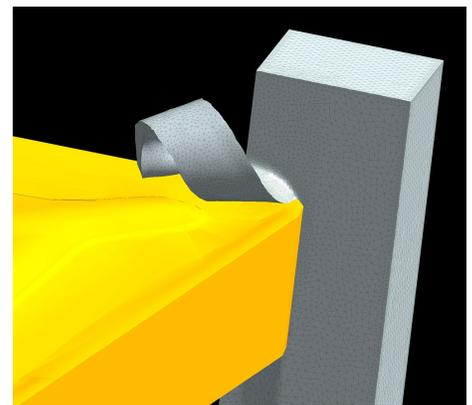
An extremely advanced, robust solver and mesh generation technology is necessary for three dimensional simulation of metal removal processes such as this drill and lathe insert. Drill geometry courtesy of WZL Aachen.
