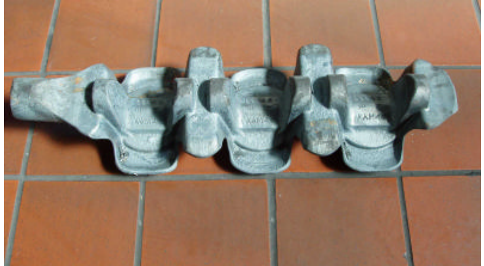
The hot forged yoke is shown prior to trimming the flash.
