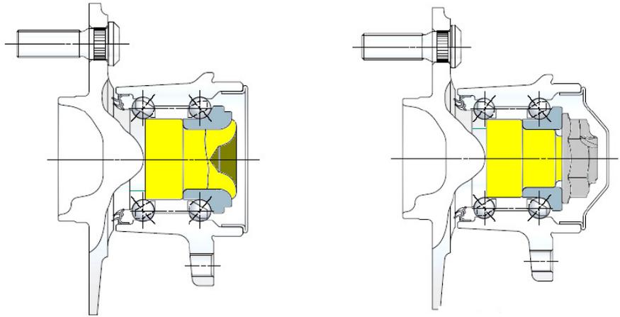
The quality of the assembly stems from the shape of the formed spindle flange. A large flange diameter will provide more contact area between the bearing race and spindle. This allows for a higher restraining force with a lower induced stress on the bearing race. Inward material flow will reduce the contact area and is undesirable. The flange geometry should sufficiently restrain the bearing race when the desired flange height is reached.
