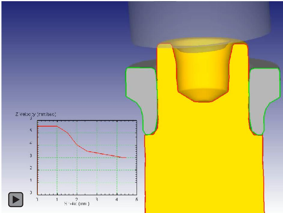
The V1 axial feed rate also decreases as the flange is formed. In this case the axial feed rate remains high enough to maintain outward flow of material throughout the process.
