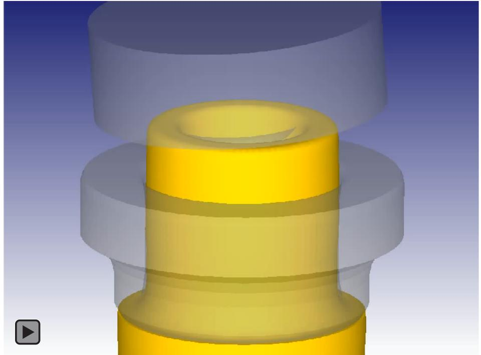
The orbital forming tool requires several revolutions to form the desired flange height.
