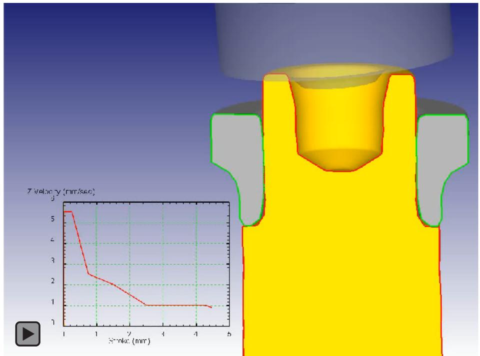
The process using the V4 axial feed rate is shown above. The axial feed rate decreases as a function of the stroke. Near the end of the stroke the axial feed rate becomes so low that inward material flow is observed.
