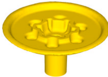
A model of the spindle is shown after the final forging operation.
