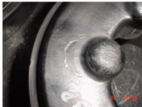
The high wear areas on the second station punch are shown (left). The wear rates predicted by DEFORM (red is higher) match the wear pattern on the punch.
