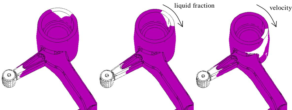
**Fig. 4:** Mould fill simulation of an experimental part.
