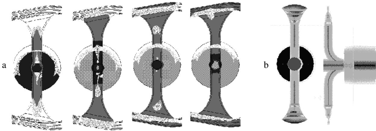
**Fig. 2:** a) Mould fill simulation with gas model. The formation of gas bubbles inside the gating system and their transport along the channel is shown.
