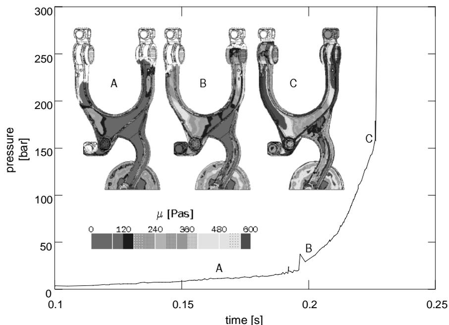
**Fig. 3:** Mould fill simulation of a thin walled component. Simulated pressure curve and local viscosity distribution during filling.
