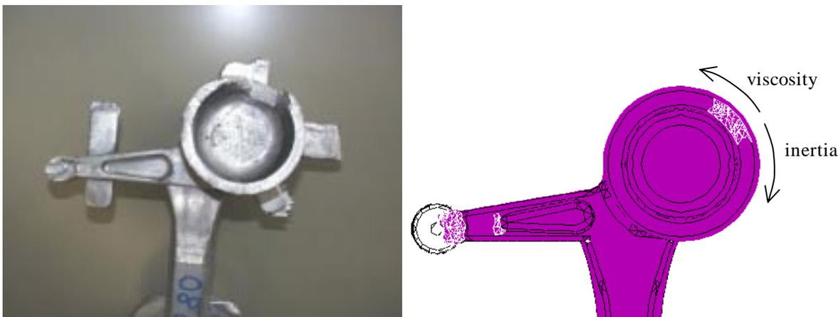
**Fig. 5:** Comparison of a fill stop of an experimental part with the simulated fill position with 40% liquid fraction and a piston velocity of 0.2m/s (The white lines show the position of the free surface).
