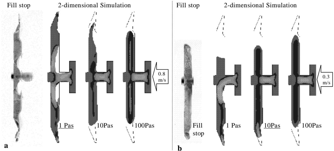
**Fig. 1:** Gating system for a 2-cavity mould. Comparison between experimental fill stops and 2-dimensional mould fill simulations using constant viscosity values.
