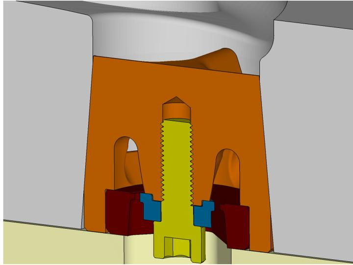
Figure 8: Cross-section through the cartridge assembly of the modified die design.
