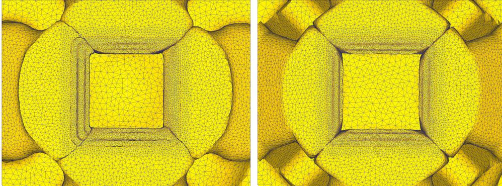
Figure 10: Weld seam locations using the original (left) and new (right) die design.
