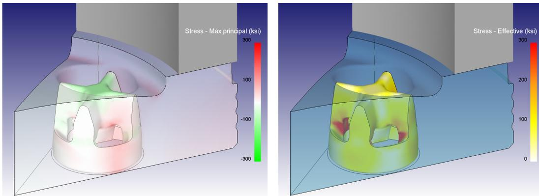
Figure 9: Locations of high principal stress (left) and effective stress (right) in the new die assembly.
