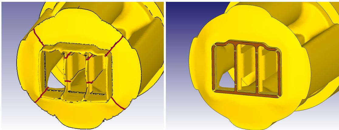
Figure 12: Weld seams predicted in Updated Lagrangian (left) and ALE (right) analyses. Both approaches show the flows merging at the same locations.
