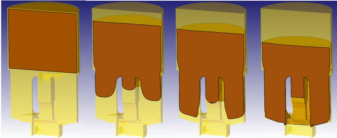
Figure 11: Sequence showing the new flownet updating in an ALE extrusion simulation.
