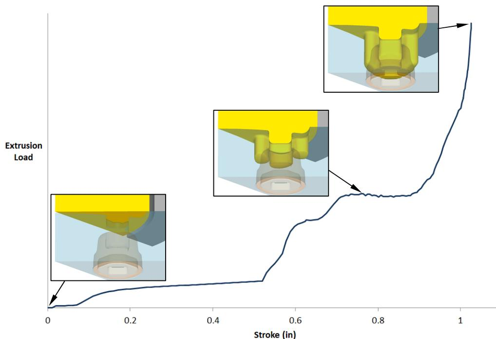
Figure 5: Load vs. stroke curve for the original die design, as well as images showing the progressing deformation.
