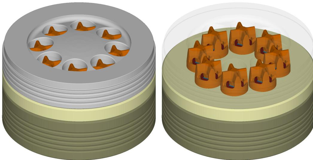
Figure 7: Modified modular extrusion die design. The bridges on the holder were removed and added to the internal cartridges.
