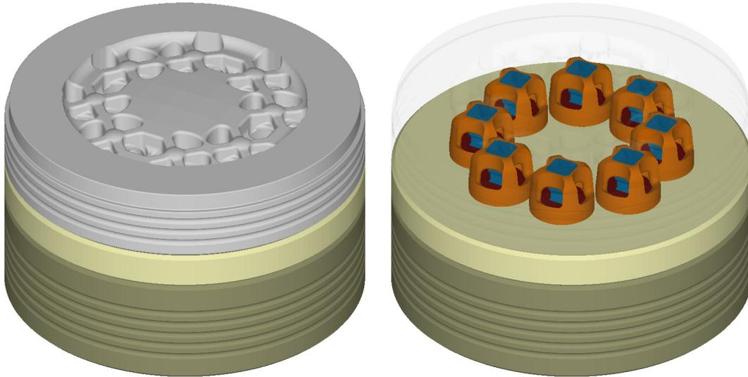
Figure 1: Original design for a modular hollow tube extrusion die. The top holder was made transparent on the right so that the internal cartridges could be seen.
