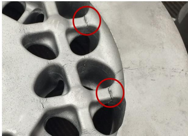
Figure 2: The holder consistently cracked at the locations highlighted.
