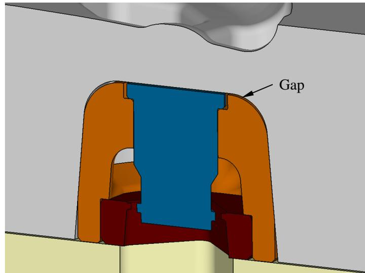
Figure 3: Cross-section through the cartridge assembly of the original die design.
