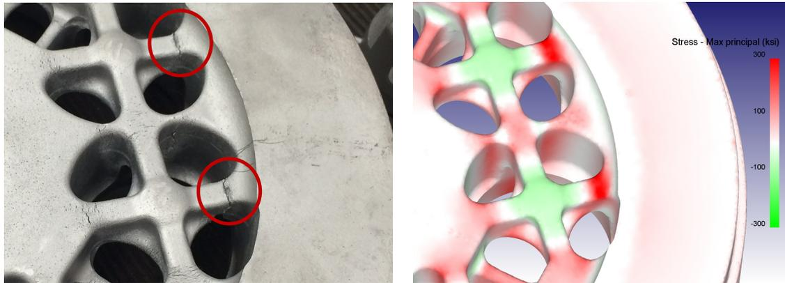
Figure 6: Locations of high principal stress (red is tension) match the cracks observed in the holder.
