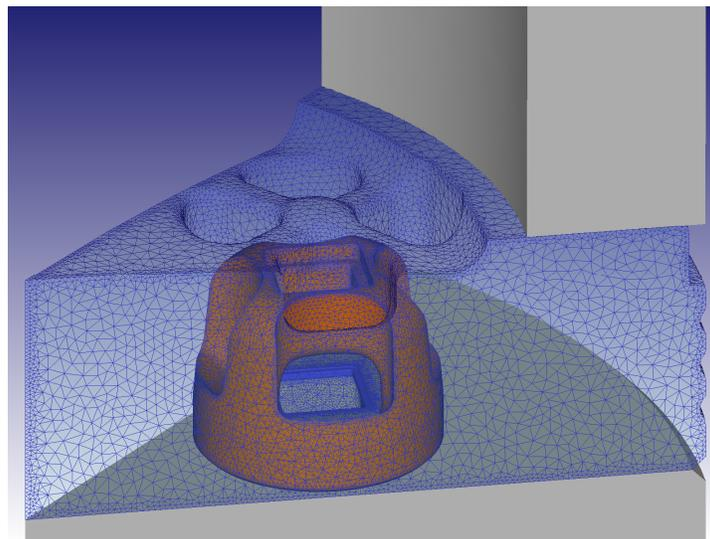
Figure 4: Mesh system used on the die components in the coupled die stress analysis.
