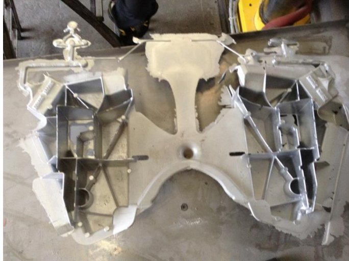
Figure 10: 2mm LPDC casting. Courtesy of FMB
