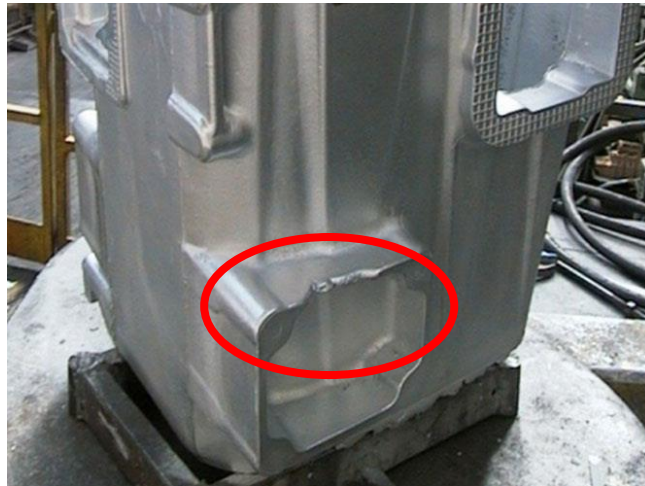
Figure 1: Example of LPDC, Low Pressure Die Casting, component without vacuum Courtesy of FMB
