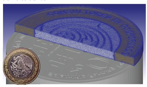
The die used in this coining process extensive engraved text and other fine details. In order to investigate the stresses in the die, a large number of elements was required. The die was meshed using 1.9 million elements. A decoupled die stress analysis was run. The image below shows the effective stress in the die (red is higher). The close-up view shows the mesh resolution in this model. Note the resolution around the text.
