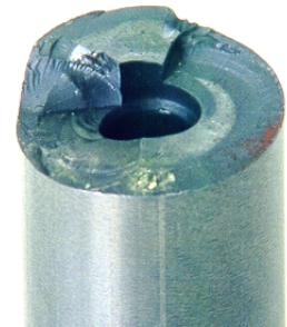
Examples of actual die insert fracture. Note the compound fracture direction, with visible fracture propagation in the axial and radial directions.
