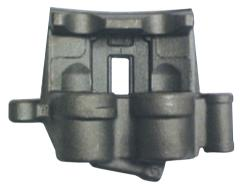
Brake calliper (GGG-50-7) with 2 cylinders. Courtesy Azterlan Research Center
