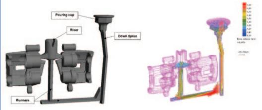
Filling System used to manufacture the part
