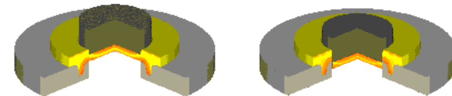
contours of temperature are shown before and after piercing operation. Note the separation of the slug from the forging (right).
