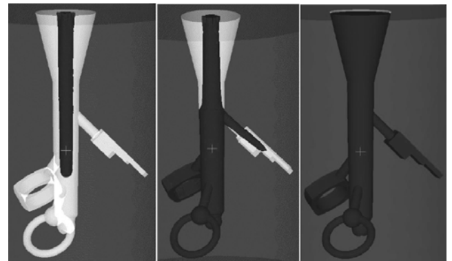
Fig. 14 The simulated filling using ProCAST
