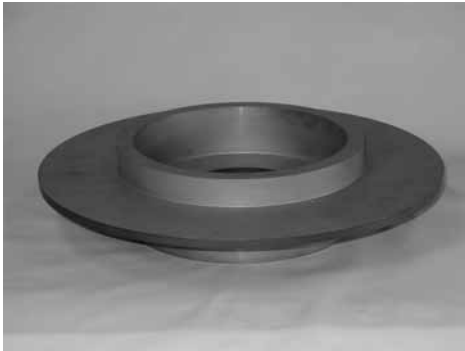
Fig. 22 Forging of U720 after all four quadrants have been machined
