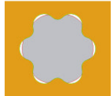
Above, a cross-section through the bearing area is shown. The underfill is visible on the corners in white.
