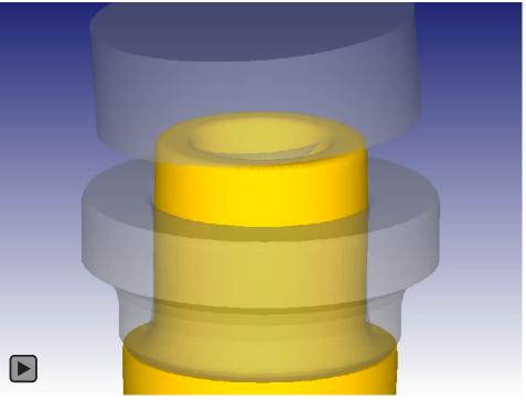
The orbital forming tool requires several revolutions to form the desired flange height.
