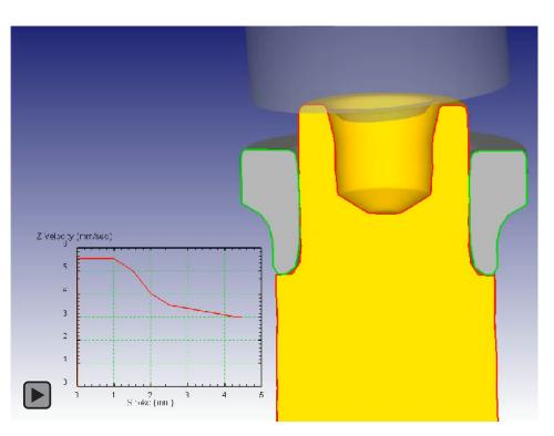
The V1 axial feed rate also decreases as the flange is formed. In this case the axial feed rate remains high enough to maintain outward flow of material throughout the process.
