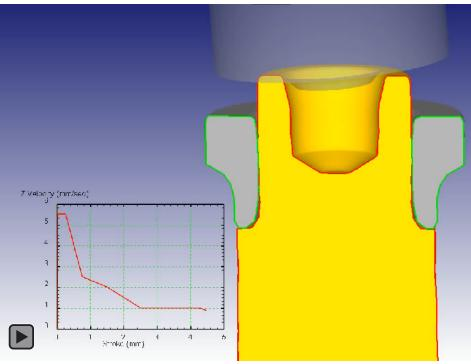
The process using the V4 axial feed rate is shown above. The axial feed rate decreases as a function of the stroke. Near the end of the stroke the axial feed rate becomes so low that inward material flow is observed.
