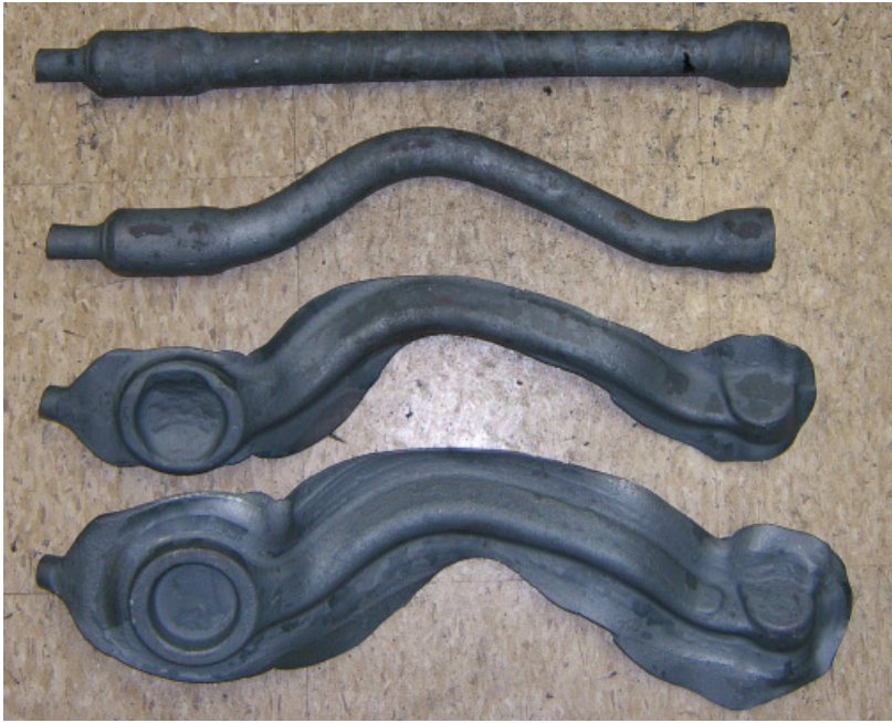
Photograph of the actual cross rolling and hammer forging outputs.
