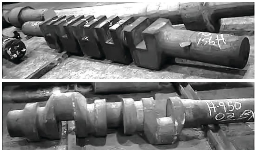
Figure 3. Large crankshafts can be manufactured using several different methods. Courtesy Ellwood Crankshaft Group
