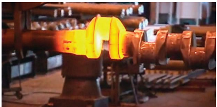
Figure 4. One method of forging crankshafts is to heat and forge the individual throws of the crankshafts to near-net shape. Courtesy Ellwood Crankshaft Group
