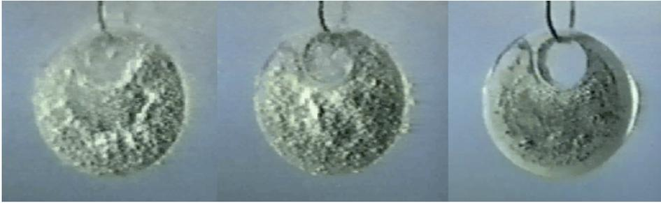
Vapor blanket formation and bubbling activity at different times during the still water quenching of the AISI-W1 steel disc component.
