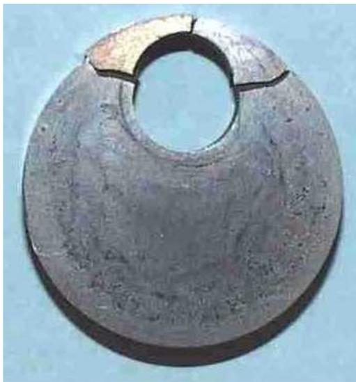
AISI-W1 component showing quench cracks (top of figure).
