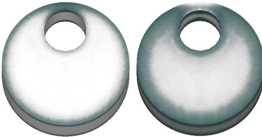
Simulated maximum principal stress in AISI-W1 component early (left) and later (right) in the quench process. Note the locations of highest stress (dark areas).
