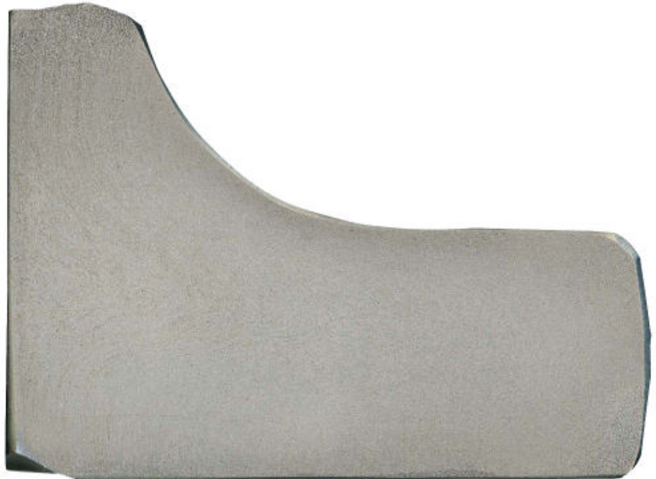
A macro section of a Waspalloy turbine disk is shown - courtesy of Carmel Forge.
