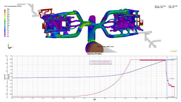
Image: Integration of Colosio Machine database & ESI ProCAST solver to achieve Real Time Piston Control
